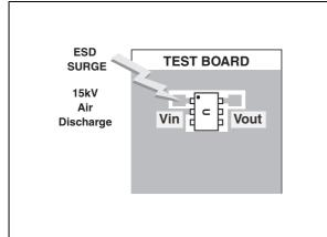
To have a good approximation of the remaining voltages at both Vin and Vout stages, we give the typical dynamical resistance value  $R_d$ . By taking into account these following hypothesis :  $R_t > R_d$ ,  $R_g > R_d$  and  $R_{load} > R_d$ , it gives these formulas:
